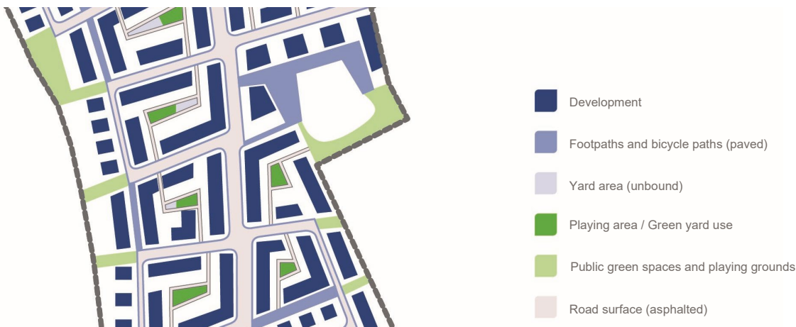
FIGURE 1 Exemplary illustration of how the areas in a district can be categorised with regard to accessibility (source: own illustration based on Faerber planning)
